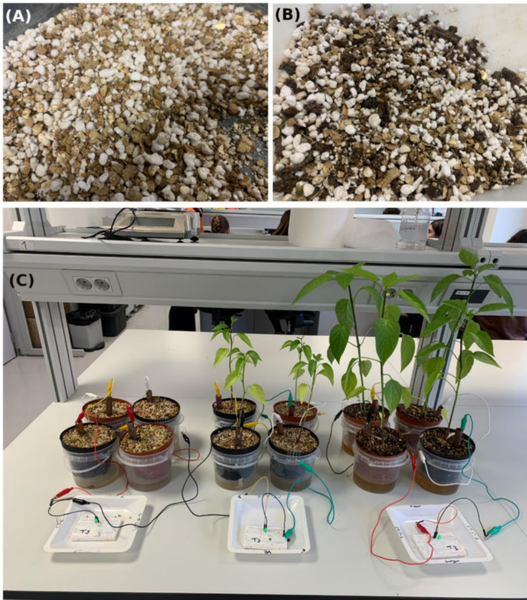
Figure 2. An overview of the plant substrates: Substrate 1, perlite/vermiculite (A); Substrate 2, perlite/vermiculite/compost (B); and the hydroponic battery-pots system used during peppers growth experiment (C).
